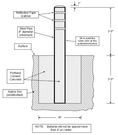
Guard post to be completely filled with concrete. 2019 CFC 312
